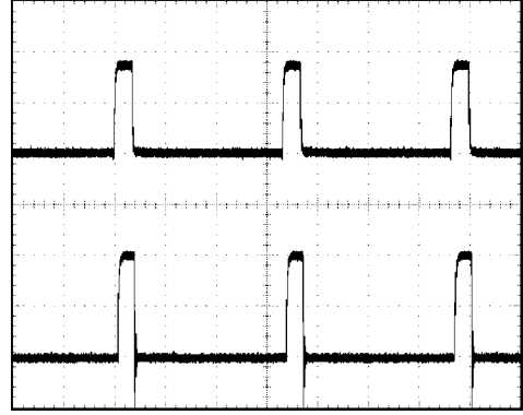
30kHz PWM Dimming (10% Duty Cycle ON)
